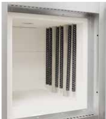
Vertically mounted SiC rods
