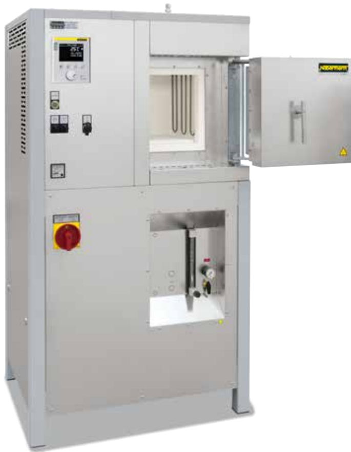
HT 16/18 with gas supply system
