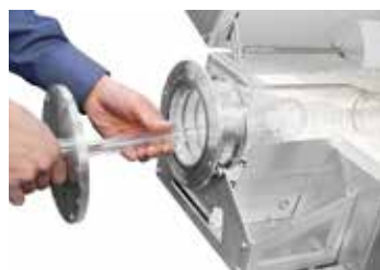
Gas tight closing plug for tubes made of silica glass closed at one side
