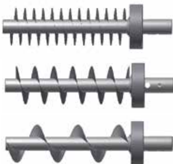
Screw-conveyors with different pitches for the adaption to the charge
