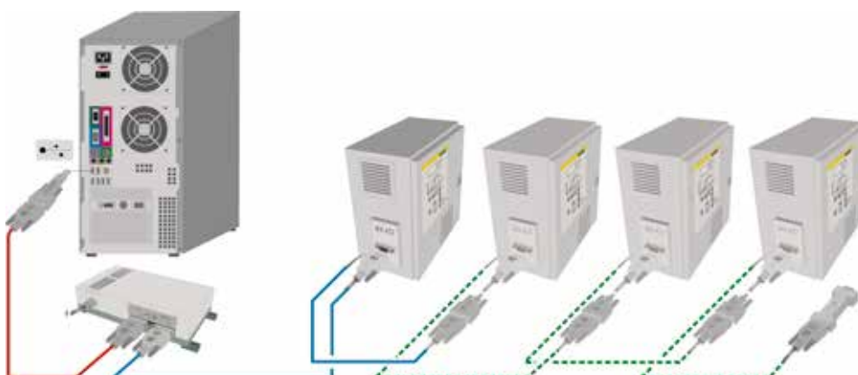
Extendable for connection of up to 16 furnaces
