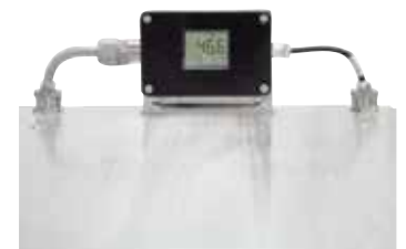
Optical temperature measurement for the use as lab strand annealing furnace
