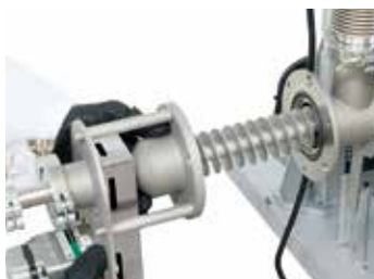
Screw-conveyor with adjustable speed
