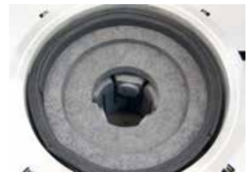
Graphite heating module
